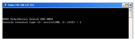
3. The Console login screen will be displayed. Press Enter to open the Account pop-up selector and then select either admin or user. Use the keyboard's down arrow to move the cursor to the Password field, enter the Console Password (this is the same as the Web Browser password; leave the Password field blank if a console password has not been set), and then press Enter.
