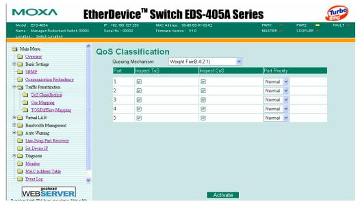
The EDS supports inspection of layer 3 TOS and/or layer 2 QoS tag information to determine how to classify traffic packets. (NOTE: The user interface for the EDS-408A shows 8 ports.)
