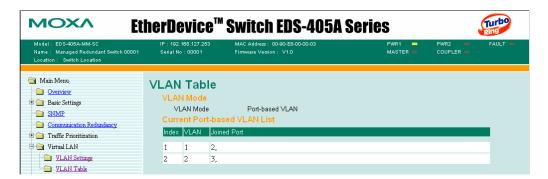
Using this table, you can review the created VLAN groups and joined ports. (NOTE: The user interface for the EDS-408A shows 8 ports.)
