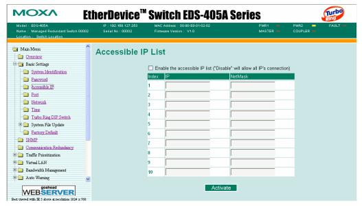
Accessible IP Settings allows you to add or remove *Legal* remote host IP addresses to prevent unauthorized access. Access to the EDS is controlled by IP addresses. That is, if a host's IP address is in the accessible IP table, then the host will be allowed access to the EDS. You can allow one of the following cases by setting this parameter
