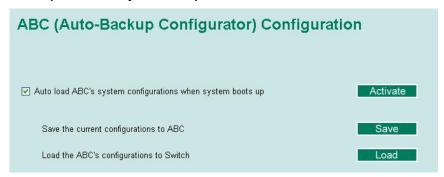
Auto load system configurations when system boots up
