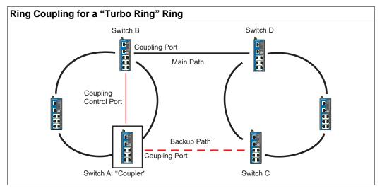
To configure the Ring Coupling function for a "Turbo Ring" ring, select two EDS units (e.g., Switch A and B in the above figure) in the ring, and another two EDS units in the adjacent ring (e.g., Switch C and D).
