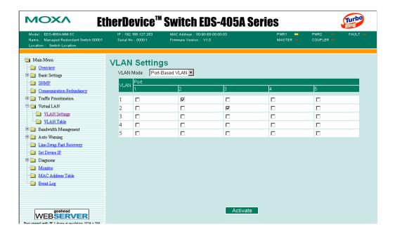
**NOTE** Port-based VLAN settings only affect one switch. The EDS-405A can have a maximum of 5 VLAN settings and the EDS-408A can have a maximum of 8 VLAN settings.
