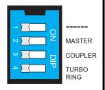
The following tables show how to use the DIP switches to configure the EDS for "Turbo Ring" or "Turbo Ring V2."
