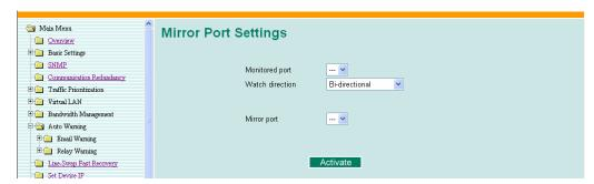
The **Mirror port** function can be used to monitor data being transmitted through a specific port. This is done by setting up another port (the *mirror port*) to receive the same data being transmitted from, or both to and from, the port under observation. This allows the network administrator to "sniff" the observed port and thus keep tabs on network activity.
