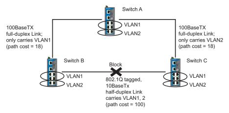
To avoid subdividing VLANs, all inter-switch connections should be made members of all available 802.1Q VLANs. This will ensure connectivity at all times. For example, the connections between Switches A and B, and between Switches A and C should be 802.1Q tagged and carrying VLANs 1 and 2 to ensure connectivity.
