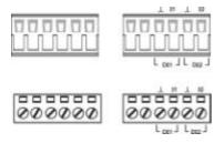
**STEP 1**: Insert the negative (ground)/positive DI wires into the /I1 terminals.
