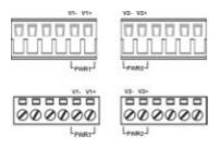
**STEP 1**: Insert the negative/positive DC wires into the V-/V+ terminals.
