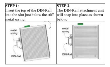
To remove EDS-508 from the DIN-Rail, simply reverse Steps 1 and 2 above.
