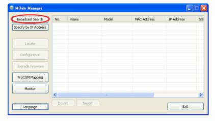
When the search is complete, every MGate EIP3000 that is found on the LAN will appear in the window with MAC address and IP address. Simply select the one that you wish to configure.
