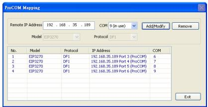
After finding the EIP3000 with the search function, select the EIP3000 device for which you want to set ProCOM for and then click **ProCOM Mapping** to enter the mapping page. Please refer to the above figures.
