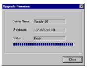
Once the downloading process ends, click on **Close** to close the Upgrade Firmware window. The **Broadcast Search** function will be activated automatically and search the LAN for all NPort 6110s.
