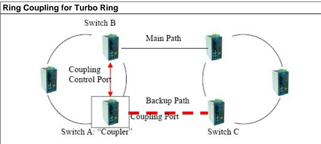
To configure the ring coupling for a **Turbo Ring**, select two PT series Ethernet switches (e.g., Switch A and B in the above figure) in the ring, and another two PT series Ethernet switches in the adjacent ring (e.g., Switch C and D).
