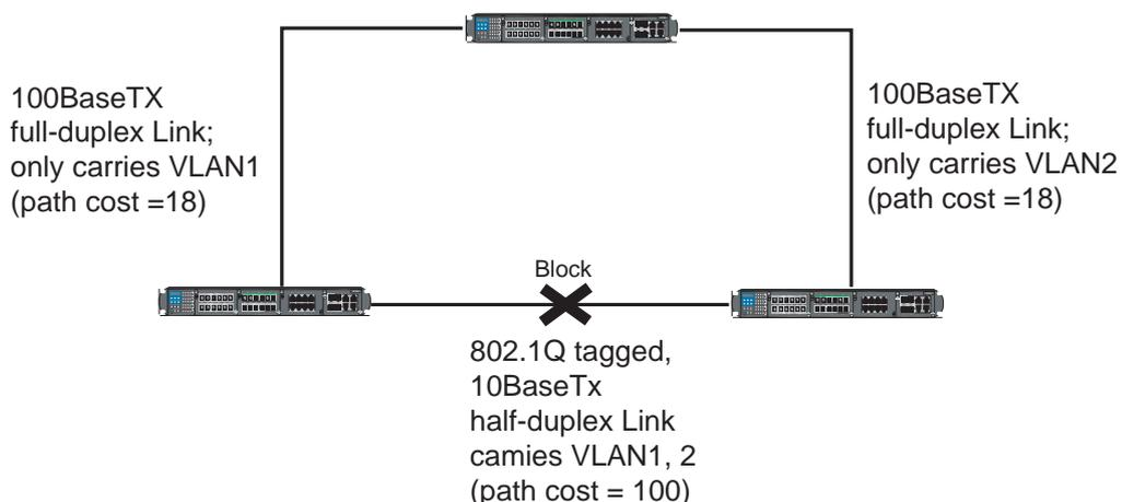
To avoid subdividing VLANs, all inter-switch connections should be made members of all available 802.1Q VLANs. This will ensure connectivity at all times. For example, the connections between Switches A and B, and between Switches A and C should be 802.1Q tagged and carrying VLANs 1 and 2 to ensure connectivity.
