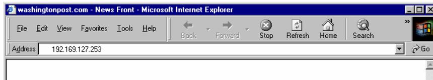
2. The PT-7728's web console will open, and you will be prompted to log in. Select the login account (admin or user) and enter the **Password**. This password will be required to access any of the consoles (web, serial, Telnet). If you do not wish to create a password, leave the **Password** field blank and press **Enter**.
