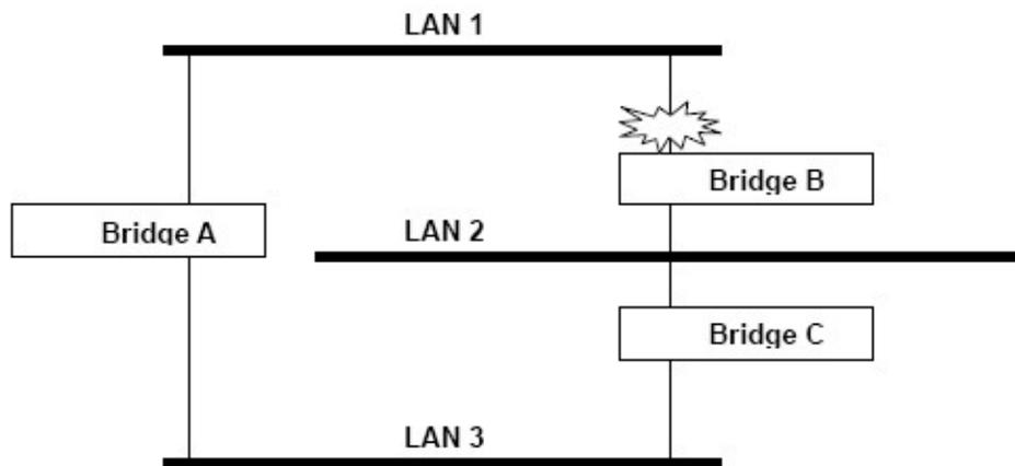
What happens if a link failure is detected? As shown in next figure, the STP process reconfigures the network so that traffic from LAN segment 2 flows through Bridge B.
