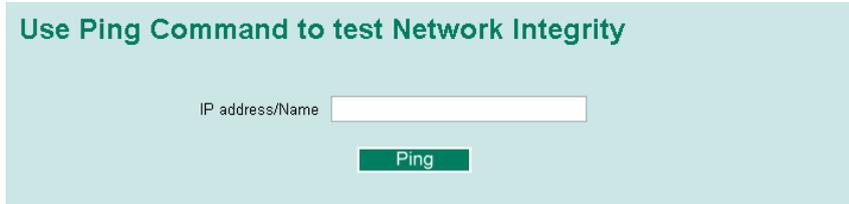
The **Ping** function uses the *ping* command to give users a simple but powerful tool for troubleshooting network problems. The function's most unique feature is that even though the ping command is entered from the user's PC keyboard, the actual ping command originates from PT-7728 itself. In this way, the user can essentially sit on top of PT-7728 and send ping commands out through its ports.
