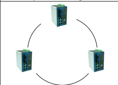
1. For each switch in the ring, select any two ports as the redundant ports.
