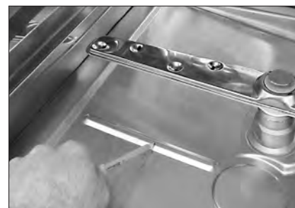
Proper Water Level in the Wash Tank.
