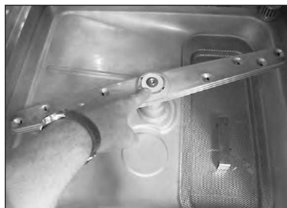
Check spray arm bearings.
