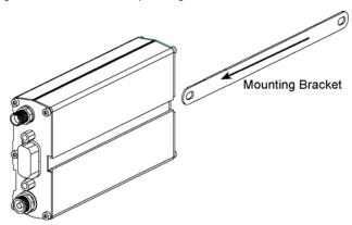
4. Attach the modern with two screws to the mounting surface at the desired location on the equipment.
