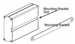
Attach the MultiModem with two screws to the mounting surface at the desired location on the equipment.
