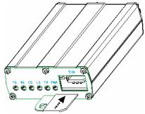
3. Verify that the SIM card fits into the holder properly and then replace the cover.
