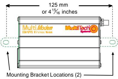
Drill the mounting holes at the desired mounting location (if applicable).
