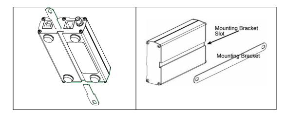
**NOTE**: Some MultiModem units will be shipped with a <u>single mounting bracket</u>. Slide it through the channel on the MultiModem chassis and secure it with screws.
