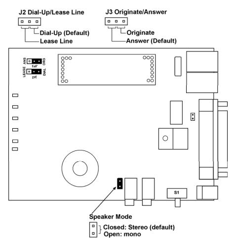
Note: The Speaker Mode Jumper is for the Modem with the Voice Option
