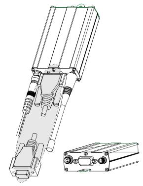
Plug the power supply cable into the wireless Multimodem. OptionalDirect DCPower Cable
