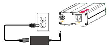
**Note:** The FF100's power supply connector will be either: (1) a plug-to-jack connection with a screw-on retaining ring, or (2) a simple plug-to-jack connection.
