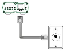
Caution: Before connecting to the Ethernet Network, make sure that the network to which you are connecting the FaxFinder is not a 192.168.2.x subnet. Because the FaxFinder's factory default IP address is 192.168.2.1, connecting it to a network that has a different device at that same IP address would cause data interference.
