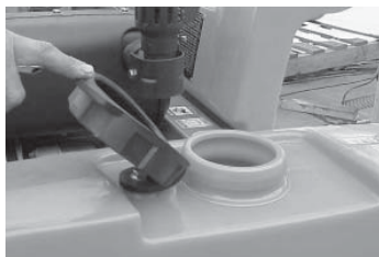
Figure 9. Checking Water Tank
