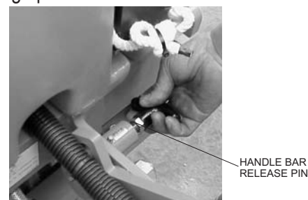
Figure 11. Positioning the Handle Bar
