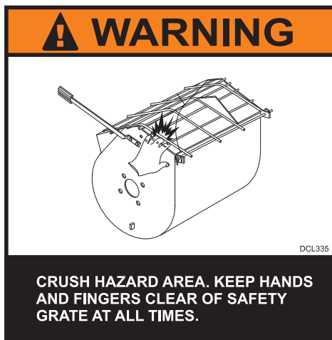
Figure 42. Safety Grate (Crush Hazard)
