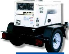
225 amp welder 6 kW AC output Kubota diesel engine SDW225SSA
