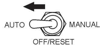
Figure 55. MPEC Control Switch (AUTO)
