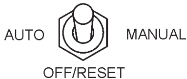
Figure 57. MPEC Control Switch (Off/Reset)
