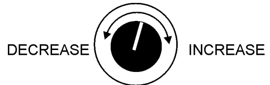
Figure 47. Voltage Adjust Control Knob
