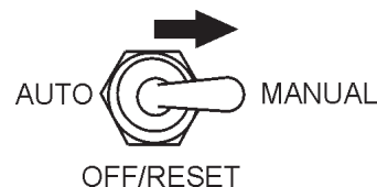
Figure 42. MPEC Control Switch (Manual Position)
