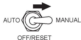
Figure 40. MPEC Control Switch (Manual Position)
