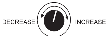
Figure 23. Voltage Regulator Knob (139V/240V)
