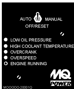
Figure 50. Engine Controller Status LED
