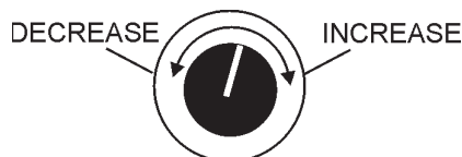
Figure 24. Voltage Regulator Knob (139V/240V)
