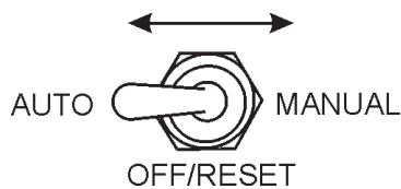
Figure 55. MPEC Control Switch (AUTO)
