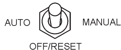
Figure 56. MPEC Control Switch (Off/Reset)
