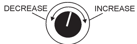
Figure 11. Voltage Regulator Control Knob
