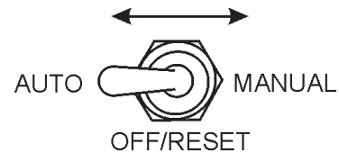
Figure 54. MPEC Control Switch (AUTO)
