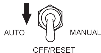
Figure 56. MPEC Control Switch (Off/Reset)
