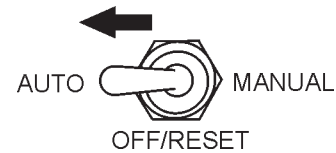
Figure 57. MPEC Control Switch (AUTO)
