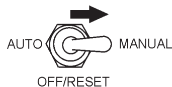
Figure 43. MPEC Control Switch (Manual Position)
