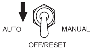
Figure 54. MPEC Control Switch (Off/Reset)
