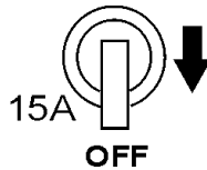
Figure 11. GFCI Circuit Breaker (OFF)
