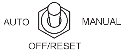
Figure 55. MPEC Control Switch (Off/Reset)
