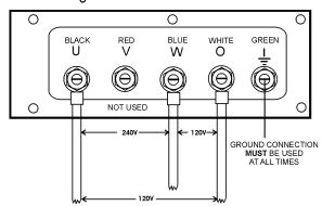
Figure 27. UVWO Terminal Lugs 1Ø-200/100V Connections
