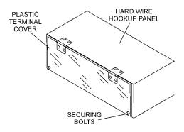
Figure 10. Plastic Face Plate (Output Terminal Lugs)
