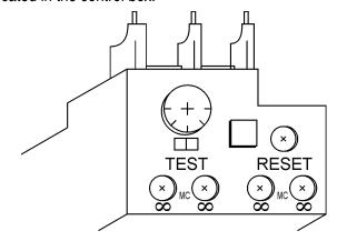
Figure 12. Over Current Relay
