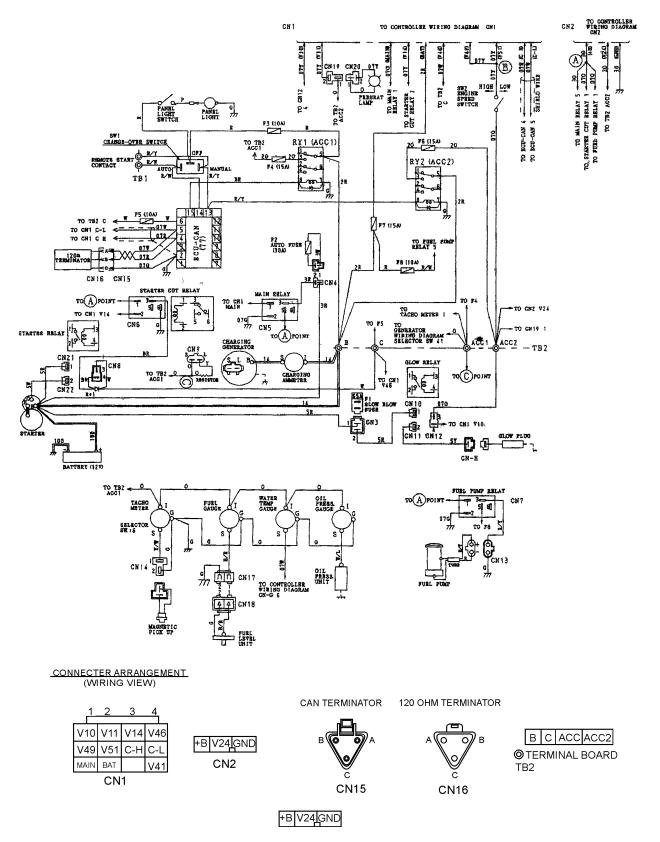
Figure 63. Engine Wiring Diagram
