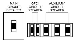
Figure 36. Main, Aux. and GFCI **Circuit Breakers (OFF)**
