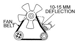
Figure 34. Fan Belt Tension
