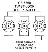
Figure 8. 120/240V Twist-Lock Auxiliary Receptacles
