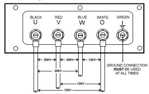
Figure 23. UVWO Terminal Lugs 3Ø-208/1Ø-120V Connections Connections
