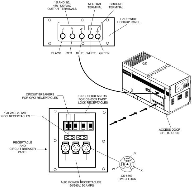
Figure 6. Output Terminal Panel
