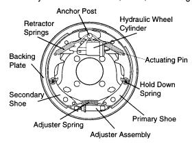
Figure 58. Hydraulic Brake Components Actuator
