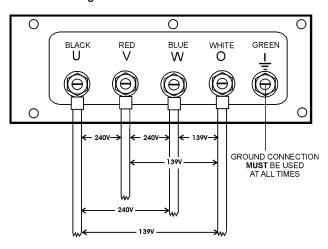
Figure 20. UVWO Terminal Lugs 3Ø-240/139V Connections
