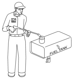
Figure 56. Fuel Tank Cleaning
