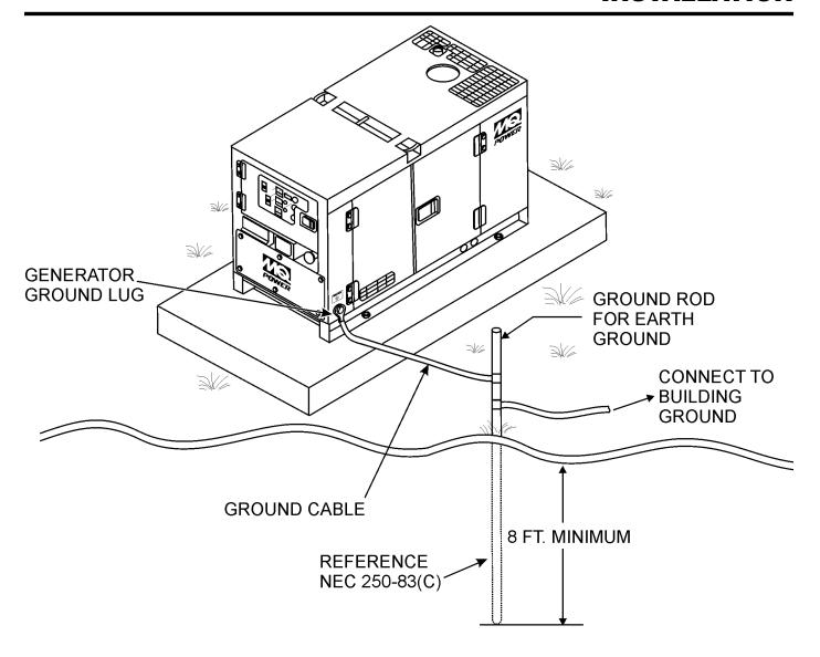
Figure 2. Typical Generator Grounding Application
