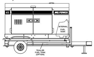
Figure 29. Internal Fuel Tank System
