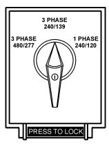
Figure 13. Voltage Change-Over Board
