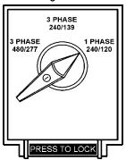
Figure 26. Voltage Selector Switch 1Ø-240/120V Position
