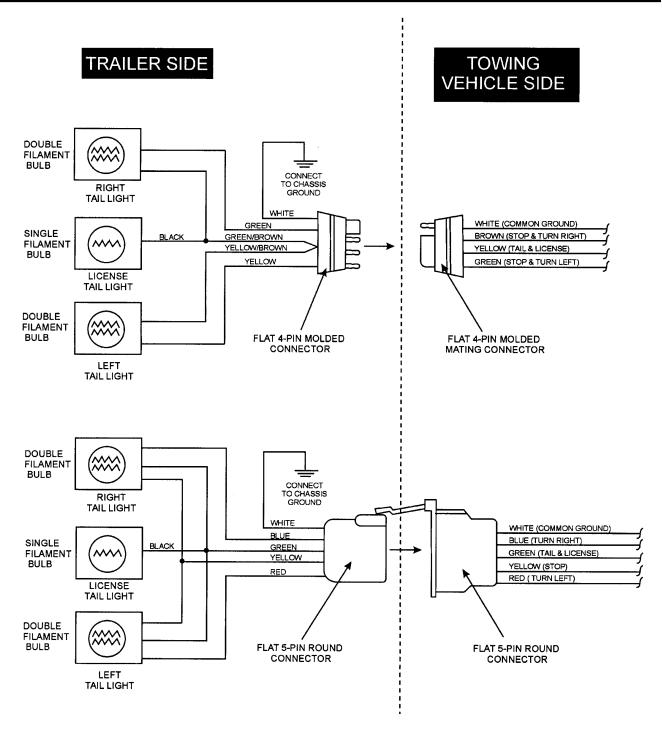
Figure 61. Trailer/Towing Vehicle Wiring Diagram
