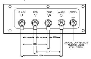
Figure 25. UVWO Terminal Lugs 3Ø-440/254V Connections
