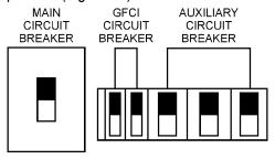
Figure 50. Main, Aux. and GFCI Circuit Breakers (ON)
