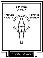
Figure 14. Voltage Selector Switch 240/139V 3Ø Positio
