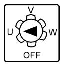
Figure 17. AC Ammeter Change-Over Switch
