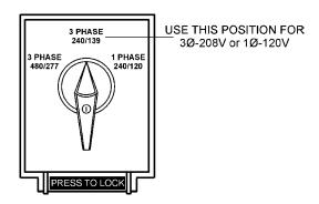
Figure 22. Voltage Selector Switch 3Ø-240/139V Position
