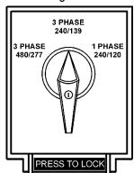
Figure 19. Voltage Selector Switch 3Ø-240/139V Position
