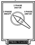
Figure 24. Voltage Selector Switch 3Ø-480/277V Position
