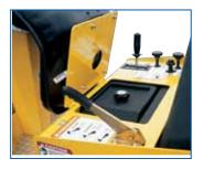
9.5-gal. fuel tank with fuel level indicator cap—located under the seat for easy access. 6.5 hours fuel supply.
