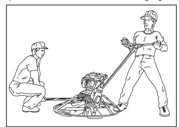
**Caution!** The machine must be stabilized by the person carrying the operator's handle. If it is not stabilized properly by this person it will rotate upside down.
