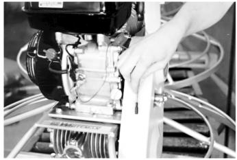
Locate the red wire protruding from the handle tube and connect it to the red wire tail on the engine. Test to insure proper operation!
