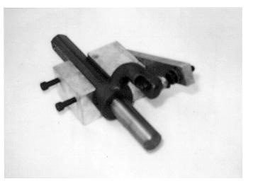
locked into the fixture, the arm bolt is adjusted to where it contacts a stop on the fixture. This will consistently adjust all of the trowel arms, keeping the finisher as flat and evenly pitched as possible. See Blade Pitch Adjustment Procedure in the Maintenance section of this manual for more information.
