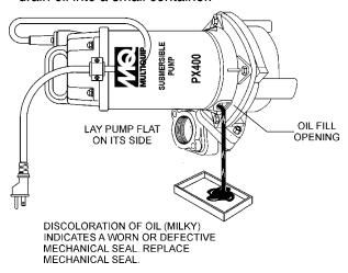
Figure 18. Draining Lubrication Oil
