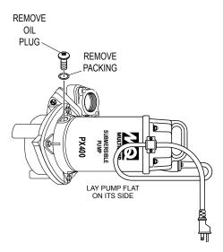
Figure 17. Checking Lubrication Oil Level
