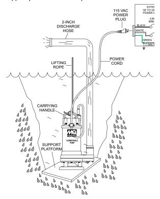
Figure 11. Submersible Pump Upright Position (Correct)
