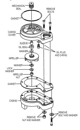
Figure 21. Mechanical Seal Impeller Removal (CX400)
