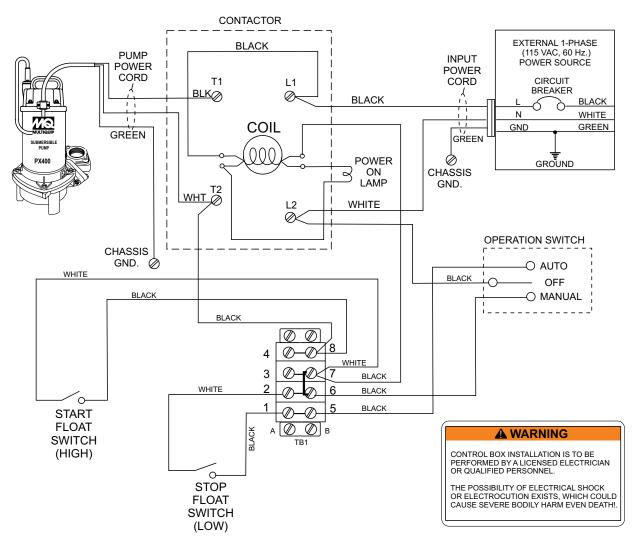
Figure 23. CB3 Wiring Diagram
