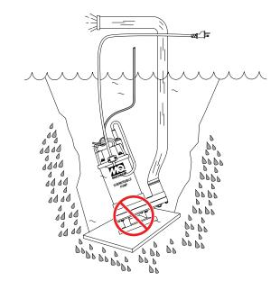
Figure 12. Submersible Pump Tilted Position (Incorrect)
