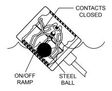
Figure 6. Float Switch (Closed)
