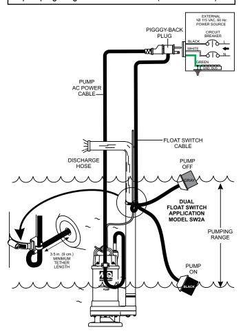
Figure 9. Dual Float Switch Application
