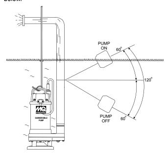
Figure 5. Pumping Range (Float Switch)
