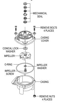
Figure 20. Mechanical Seal Impeller Removal (PX400)
