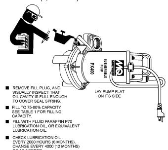
DISCOLORATION OF OIL (MILKY) INDICATES A WORN OR DEFECTIVE MECHANICAL SEAL.
