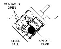
Figure 7. Float Switch (Open)
