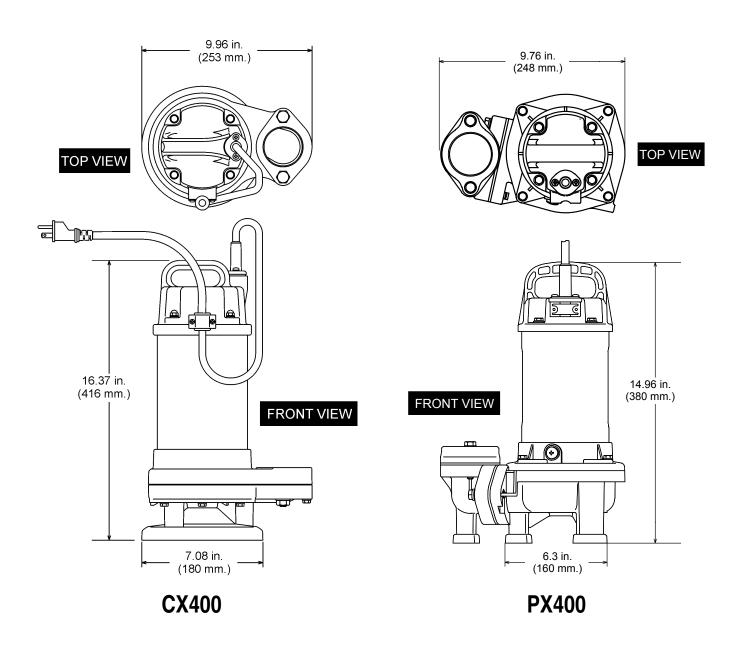
Figure 1. CX400/PX400 Pump Dimensions
