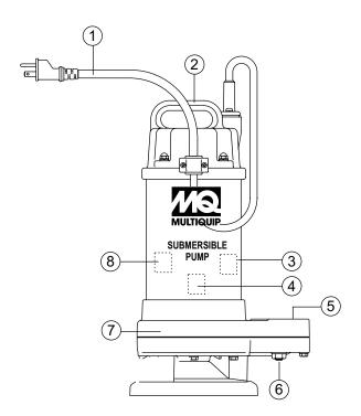
Figure 3. Submersible Pump Components
