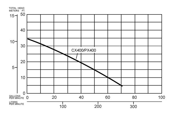
**Figure 2. Pump Performance Curve**
