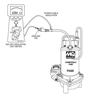
Figure 22. Insulation Tester Application
