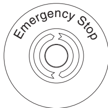
Figure 19. Emergency Stop Switch
