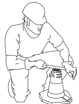
Figure 68-D. Slump Test (Removing Excess Concrete)
