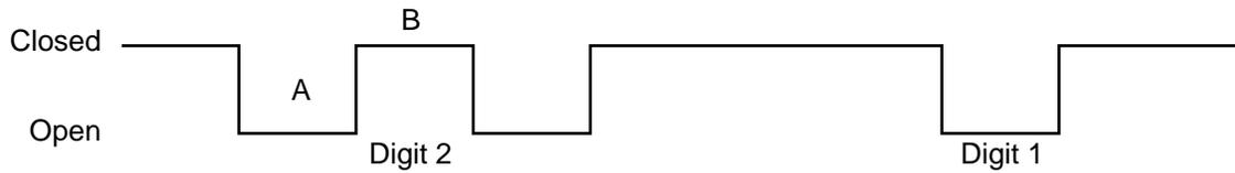
In the example above, the digit 2 is pulse dialed, followed by the digit 1. Each pulse consists of an A mSec. open and a B mSec. closed, where A will be either 60 or 67 mSec and B will be either 40 or 33 mSec., for a total of 100 mSec. per pulse, or a rate of 10 pulses per second. The interdigital pause time is 800 mSec. The pulse ratios are controlled by the **&P** command.
