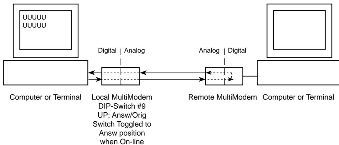
Figure 8-7. Synchronous Mode Digital Loopback Test (remote/automatic)
