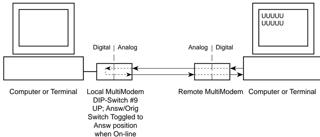
**Figure 8-6. Synchronous Mode Digital Loopback Test (local/manual)**
