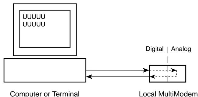
**Figure 8-5. Synchronous Mode Local Analog Loopback Test**
