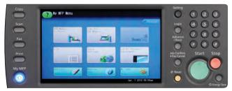
The MFX-2590 features an 8.5" color touch screen that quickly guides users through machine programming, job execution and troubleshooting. Using the illuminated keys on the control panel users can effortlessly toggle between modes, view job status, change settings, adjust the screen view and more.
