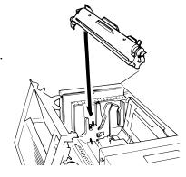
Unpack the toner cartridge from its carton. Hold the toner cartridge with both hands, and shake it well as shown.
