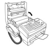
**3** Grab the handles on each side of the ink film cartridge, and lift the cartridge straight up out of the machine.
