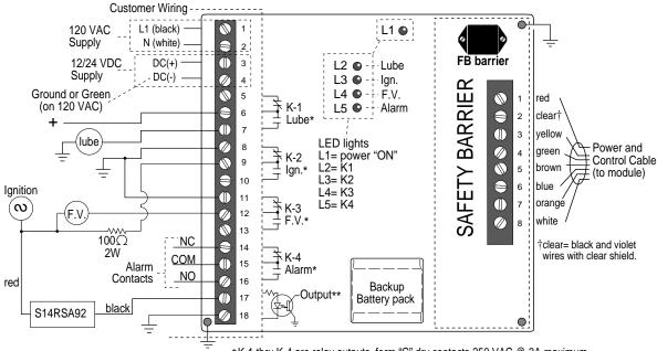
\*K-1 thru K-4 are relay outputs, form "C" dry contacts 250 VAC @ 3A maximum.
