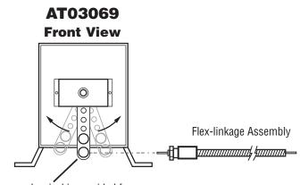
A second swivel is provided for use on the butterfly valve lever arm.
