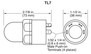
**Mounting Hole:** 1-1/8 in. (29 mm) diameter **Maximum Panel Thickness:** 1/4 in. (6 mm)
