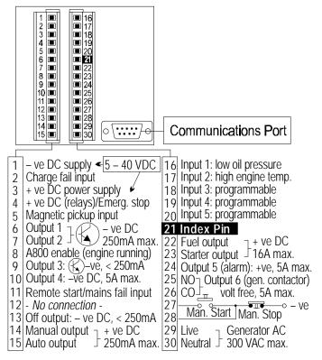
For a typical connection circuit, please see Autostart 710 data sheet (the Autostart 705 and 710 are pin compatible).
