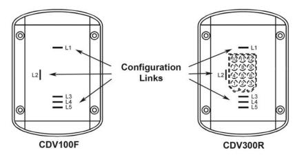
The links allow configuration of operating options by snipping the appropriate wire according to the following configuration table.
