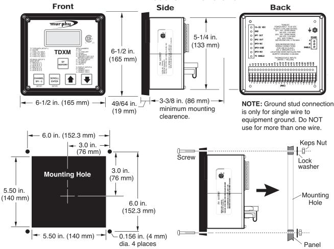
For Outdoor Use, the TDXM should be mounted in a weatherproof enclosure
