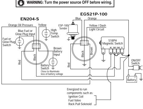
Note: Use of the black wire on the EN204-S and the 518PH Magnetic Switch (as shown in the diagram) is required for engine shutdown.
