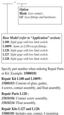
*15000180:* Includes case, contact, 4 mounting bolts, and 2 gaskets. *15000181 (L127 only):* Includes 4 mounting bolts, 2 gaskets, float assembly, ground strip, wire, and mounting plate.
