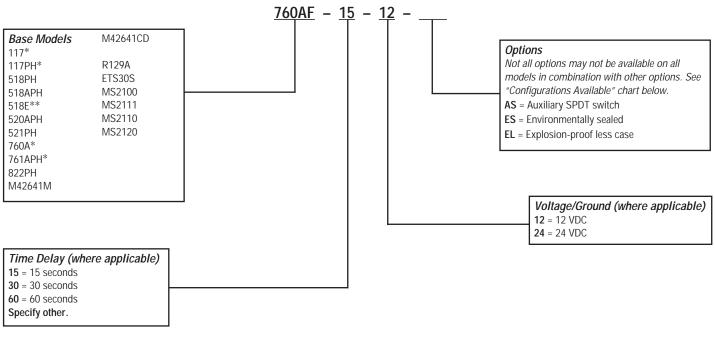
\*Add the letter "F" to the base model to indicate an inline fuse instead of a base mounted fuse. Example: 760AF, 761APHF, 117F. \*\*12 Volt negative ground version only.
