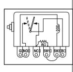
**518APH** Allows for SWICHGAGE<sup>®</sup> and/or N.C. contacts to be wired "Closed Loop" (in series). Any contact open or SWICHGAGE<sup>®</sup> contact close in the circuit shunt trips the 518APH. Specify 12 or 24 VDC. Contacts 10 amps 24V. 14 amp fuse.
