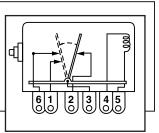
**MS2100** Multi purpose TATTLETALE® with dry contacts that can be used to make two circuits and break another when tripped. Operates from 120 VAC or Capacitor Discharge Ignition. The operating coil is intermittent duty and must be disconnected by an external circuit when tripped. The MS2100 is a replacement for 100PH, 307CD, 307PHCD and 224CD.
