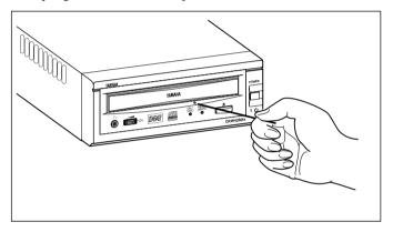
After manually ejecting a disc, you must turn off the power supplied to the CRW4260tx, then turn it on before continuing.
