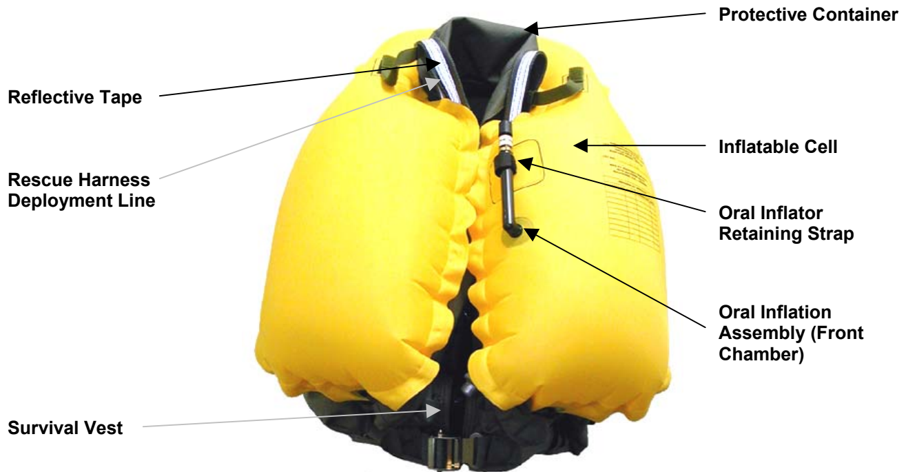
Figure 7. Component Locations – Inflated Cell
