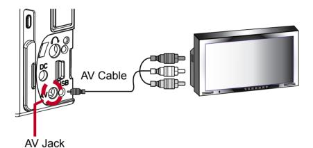
2. Connect yellow end of the cable to the Video input (yellow) jack on
