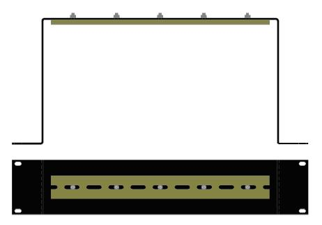
Most N-Tron<sup>TM</sup> products are designed to be mounted on industry standard 35mm DIN rail. However, DIN rail mounting may not be suitable for all applications. Our Rack Mount Assembly (P/N: 900-RM) may be used to mount the 105TX/FX-POE enclosures to standard 19" racks as an option.
