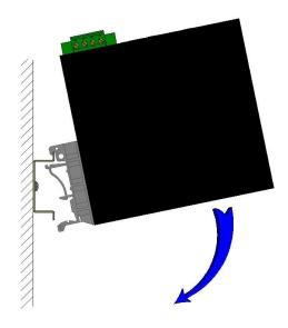
To install the unit to 35mm industrial DIN rail, place the top edge of the included mounting bracket on the back of the unit against the DIN rail at a 15° angle as shown. Rotate the bottom of the unit to the back (away from you) until it snaps into place.
